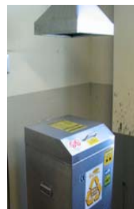
The distillation apparatus for recycling acetone effluent.
