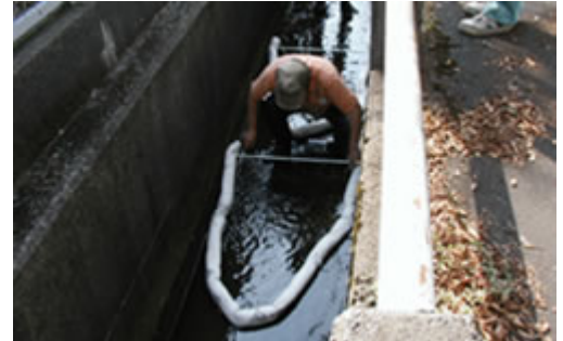
Verifying response and measures practicality and efficiency for a hypothetical spillage of heavy oil at our Nagaoka Plant (Niigata Prefecture)
