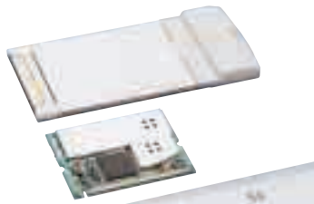
COMMUNICATION MODULE FOR IEEE 802.11a/b Combination-type for IEEE802.11a and IEEE802.11b high-speed wireless LAN standards
