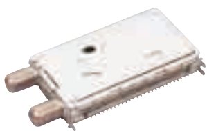
TUNER UNIT FOR DIGITAL TERRESTRIAL BROADCASTING Industry's smallest size tuner with internal demodulators compatible with broadcasting systems in Japan, the U.S. and Europe
