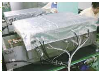
Insulation cover for drying-furnace (at Tianjin Alps Electronics, China)
