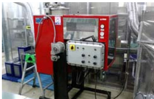
IPA effluent distillation equipment
