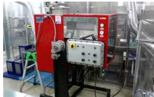
IPA effluent distillation equipment
