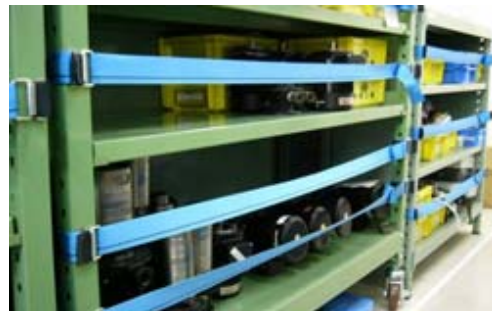
Earthquake measure 1: Items are prevented from falling off shelves
