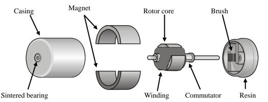
\*Pay attention to flame retardant in resin, special metals (alloys) intended of electrical properties and lubrication of commutator, and grease in sintered bearing. Calculate content amounts in respective positions, such as the case including lead wire and electronic circuit.
