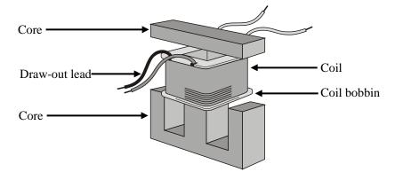
\* Pay attention to resin material, flame retardant in insulating parts, impregnant in coil, PVC and flame retardant in lead wire cover.
